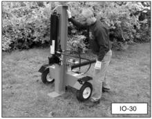
c. Turn the spring-loaded locking lever knob until the pin slides into the slot. This allows the plunger to snap into place, securing the rail assembly in a vertical position.
