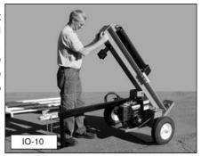
**9.** Link the ends of the safety chains to the safety quick-links and tighten the link's locknut securely with a wrench.
