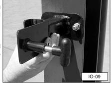
8. Block the wheels to prevent the base unit from moving. Carefully lower the rail assembly to a horizontal position. Securely tighten the nuts holding the base unit to the rail assembly (Step 5) and the nuts holding the rail rest assembly (Step 6).
