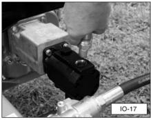
16. Remove the oil filter from the plastic cover and apply a thin coat of oil to the rubber seal. Screw the filter onto the filter head located near the hydraulic tank. Once the filter makes contact with the filter head, turn it an additional 3/4 turn. Hand-tighten only.
