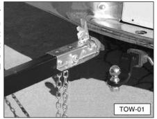
Release the latch assembly on the hitch coupler and lock the hitch coupler onto the tow ball. Attach the towing safety chains to the tow vehicle.
