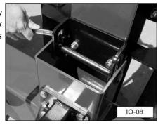
Bolt the rail rest to the rail assembly using two 1/2-13 x 1-1/2 inch long hex head bolts, lockwashers, and nuts, as shown. Hand tighten the nuts.
