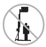
Do not stand under the load. The safety brake system (if equipped) will allow the load to drop 1 to 3 feet / 30 to 91 cm before locking the columns.
