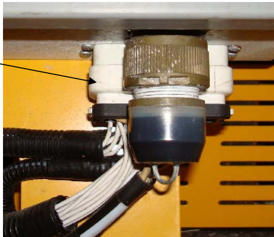
Figure 7-3. Ground Control Panel Receptacle
